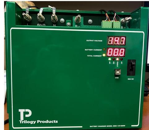
A USB and ENET Port are provided. These ports, along with a MicroSD card, real-time clock, and super capacitor, allow for a built-in data logger. Algorithms can include date and time stamping of power failures, time on AC vs. battery, charging time once AC returns, etc. A PC application that runs on any computer allows the user access to the charging system parameters and monitors the charger in real time.
