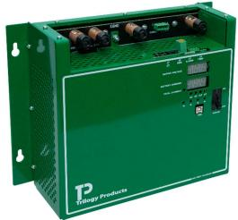
An integrated menu system uses the 7-segment displays and 4 buttons on the front panel to permit configuration and diagnostics of the charger, including setting up battery configuration and type, entering IP settings, and setting the charger's realtime clock.
